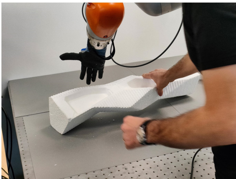
Figure 14: Assembly Process of the robotically milled Voronoi fragments
